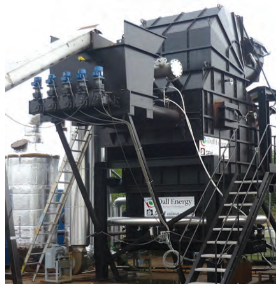
The "proof of concept" 2 MW two-stage biomass gasification pilot furnace at SEM Steel Industry. It has since been shipped to Warrick Mills, USA
