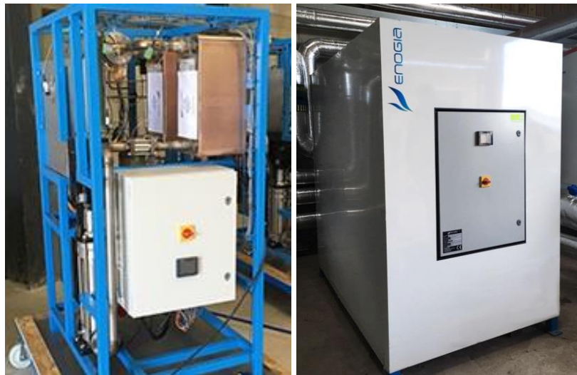
Figure 32: Commercial systems developed by Enogia: on the left, a 10 kW el generator "unboxed", on the right a 40 kW el generator completed
