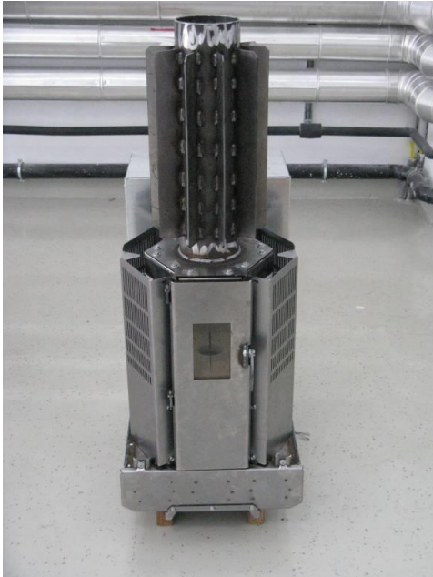
Pellet stove with TEG 400 (dummy) [102]
