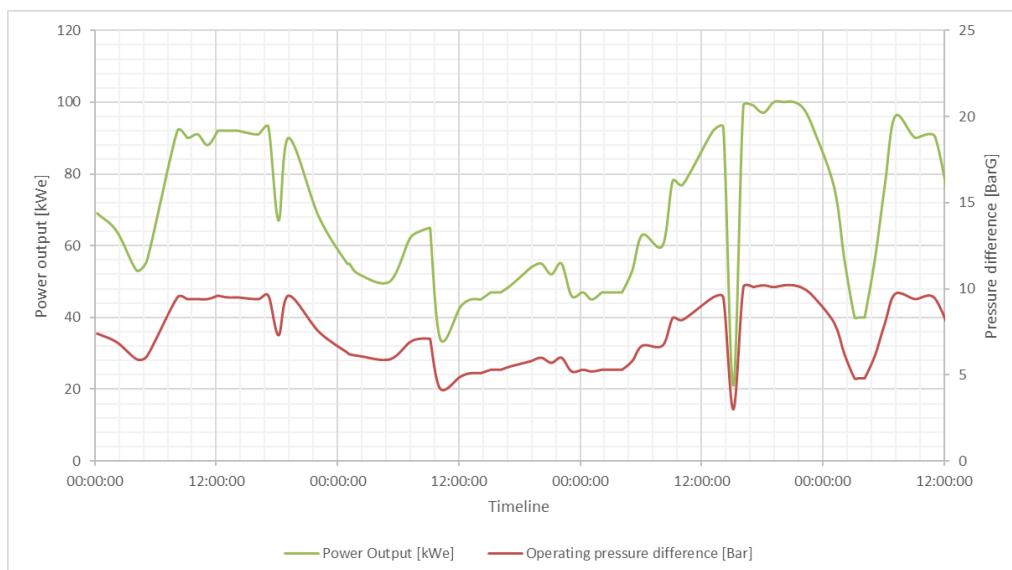
Figure 27: correlation between the power output and the pressure difference measured in 3 days of operation at a genset installed at a district heating scheme
